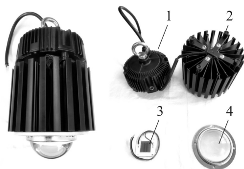
Fig. 1. Design and components of the spectrum corrector: 1 – driver, 2 – heat-sink, 3 – LED matrix, 4 – lens
